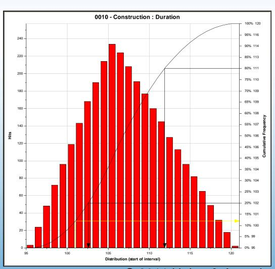
Schedule inaccuracy operates in 100% of the time (all iterations). On a construction activity of 100 days duration the results are triangular The construction labor productivity risk would look similar to this figure
