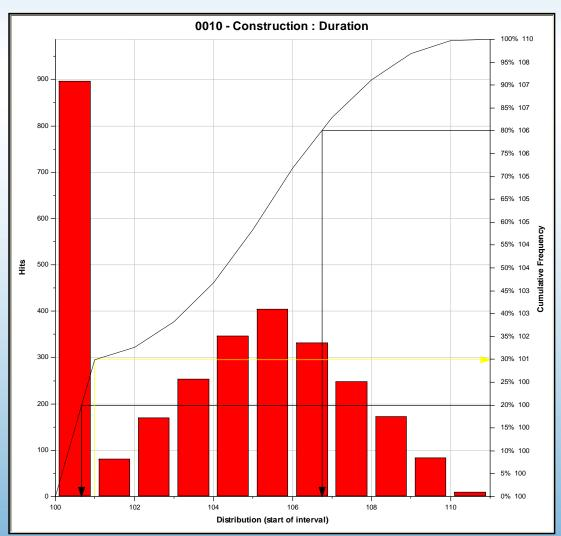
Here a risk event, the possible unavailability of quality key staff, occurs 70% of the time. Hence, in 30% (900) of the 3,000 iterations the original duration of construction, 100 days, is correct. In 70% (2,100) of the iterations, the duration is longer than 100 days as a triangle
